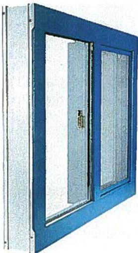
**New windows** will be dual glazed and include low E glazing where appropriate. Acceptable commercial aluminum window frame systems can be provided by EFCO, Torrence, Kawneer, Milgard or an acceptable equal. New window systems are not required to be thermally broken. ¼" glass should be specified.
