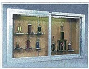
Provide Display/Bulletin Board cases at classroom building hallways and at other areas, such as the administration building, performing art centers and gymnasiums as approved by the District. These cases are to be constructed of anodized aluminum extrusions. All cases should have sliding or hinged doors and tempered glass. Provide tackable back panels and lighting.
