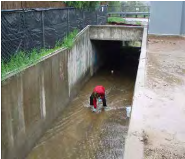
Figure 9-6. Grab Sampling at Mid-Stream, Mid-Depth
