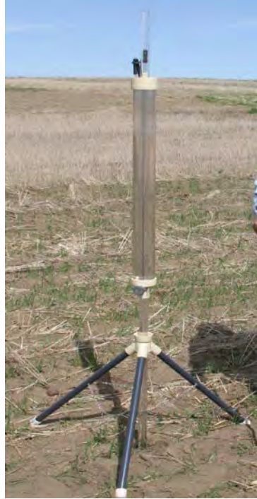
Figure C-3: Guelph Permeameter for Shallow Borehole Permeability
